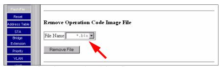
Figure 24: Removing an operation code image file
